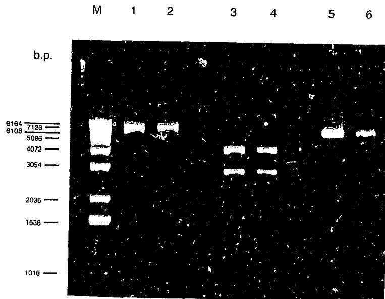
**Figure 2.** Characterization of plasmids pOHB 27-1 and pOHB 27-2. Lane M contains DNA markers. The size of the markers in base pairs (bp) are given on the left side; lanes 1 and 2 contain plasmids pOHB 27-1 and pOHB 27-2, respectively; lanes 3 and 4 contain *Eco*R1 digested pOHB 27-1 and pOHB 27-2, respectively; lanes 5 and 6 contain *Xba*I digested pOHB 27-1 and pOHB 27-2, respectively.
