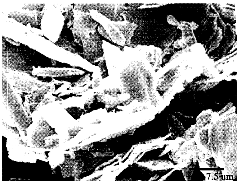
Figure A8 – SEM of Poly(2-ethylaniline)/FeOCl (2000x)
