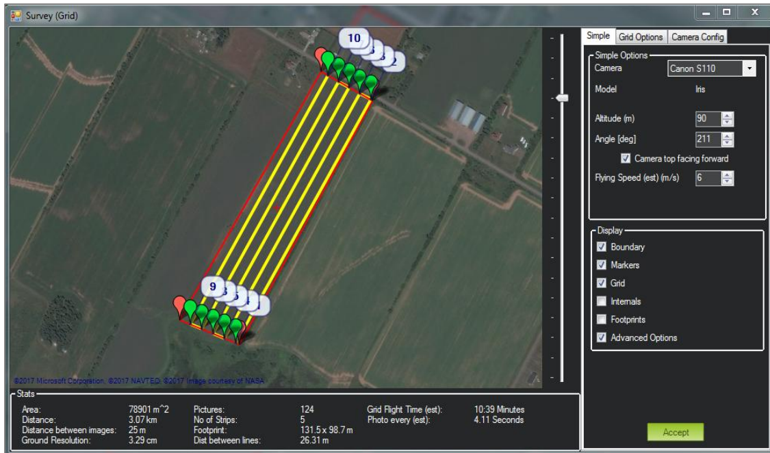
Figure 8: Mission Planner flight control software
