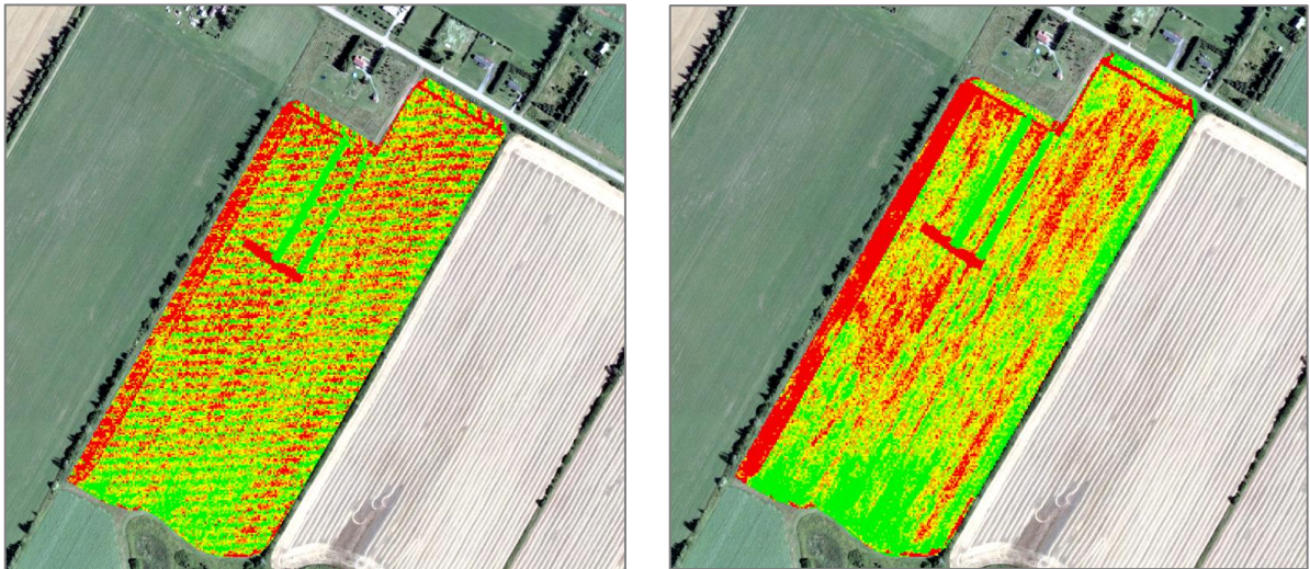
Figure 20: Bilinear Interpolation (left) vs Aggregated resampling method (right)
