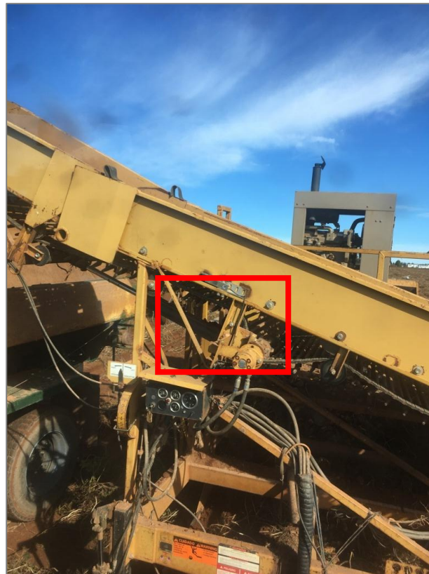
Figure 18: Greentronics yield monitor load cells and speed monitor on the harvester
