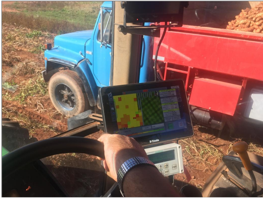
Figure 17: Greentronics yield monitor controller and interface in the tractor
