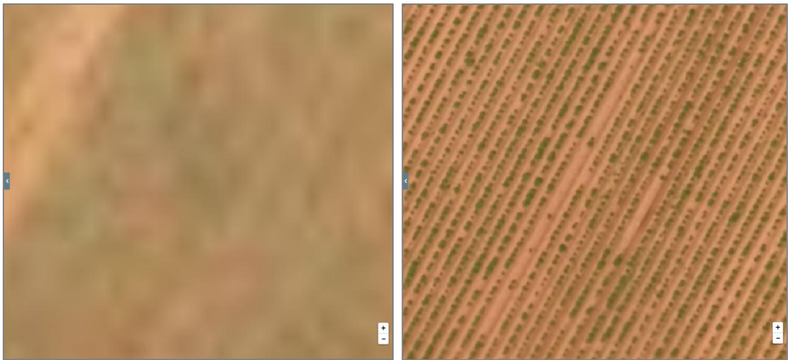
Figure 1: Example of Satellite (left) vs sUAS (right) imagery resolution. Satellite imagery courtesy dronedeploy.com
