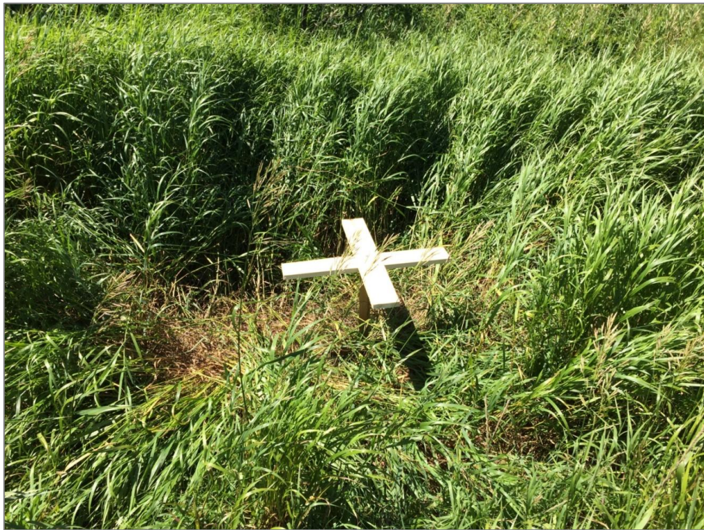
Figure 9: Image of GCP at one corner of the survey area
