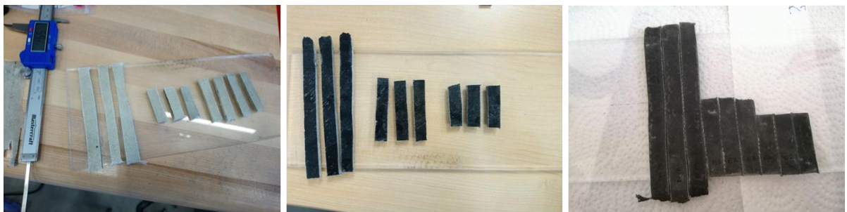
Figure 3.3: Specimen of GFRP without biochar (left), with 10% biochar (middle) & 5% biochar (right).
