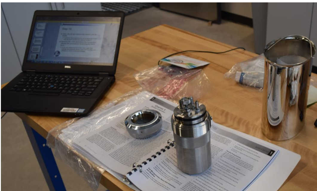
Bomb for Bomb Calorimetry Analysis being prepared.
