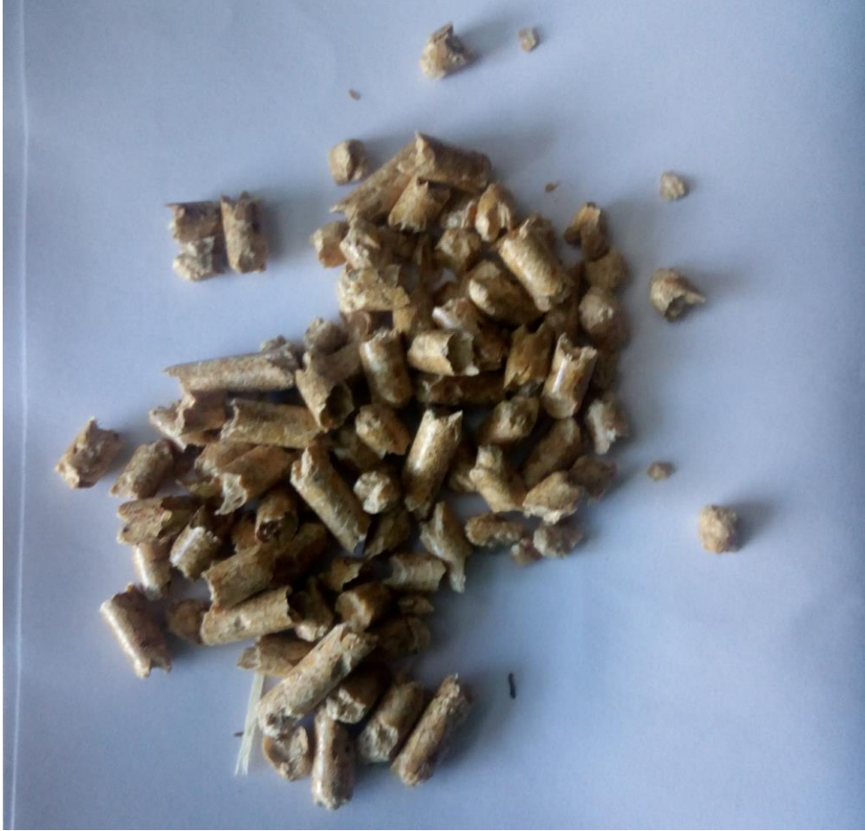
Spruce pellets pyrolysis feedstock for char production for composites application.
