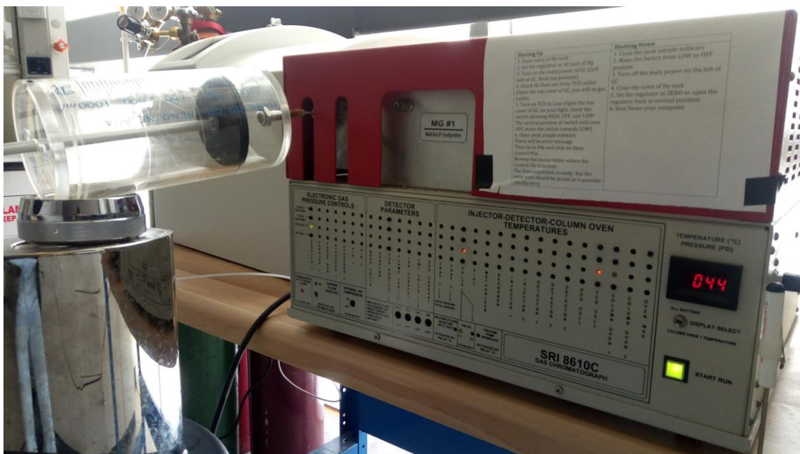
Gas analysis being performed in Gas Chromatograph.
