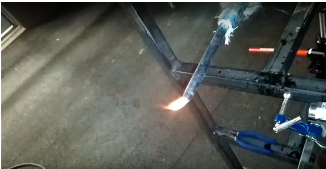
Igniting Syngas showing good combustibility.
