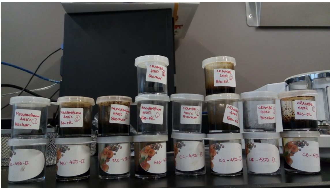
Collection of produced pyrolytic products for analysis.
