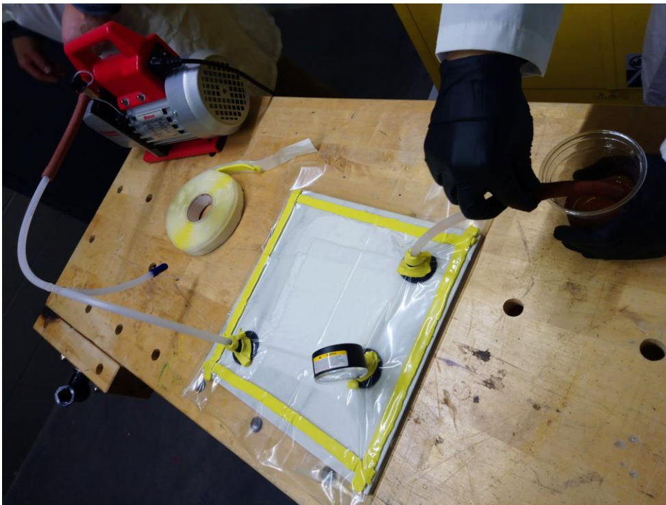
Vacuum infusion technique being applied to produce composites material.
