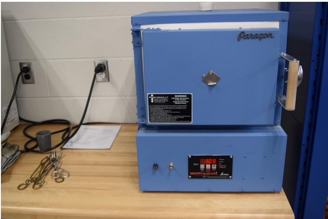
Muffle Furnace running Proximate Analysis.
