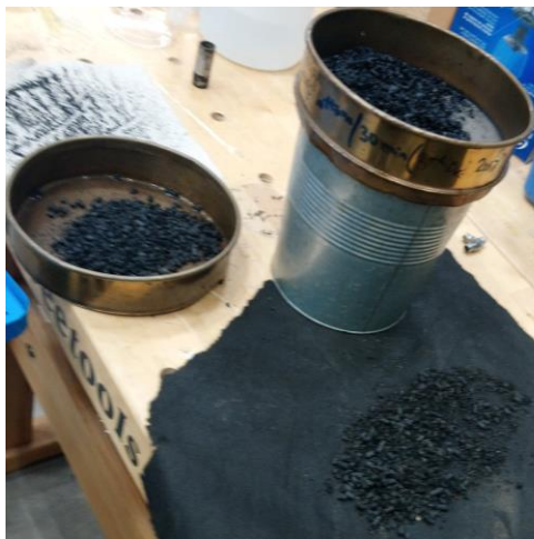
Grinding and screening of produced biochar for biocomposites application.
