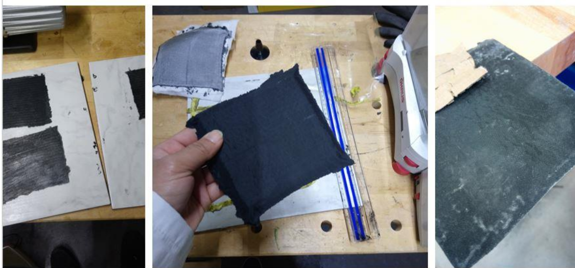
Composites samples being cured (Left), A cured Sample (Centre) & Sample held in vices to be cut in sizes for analysis (Right).
