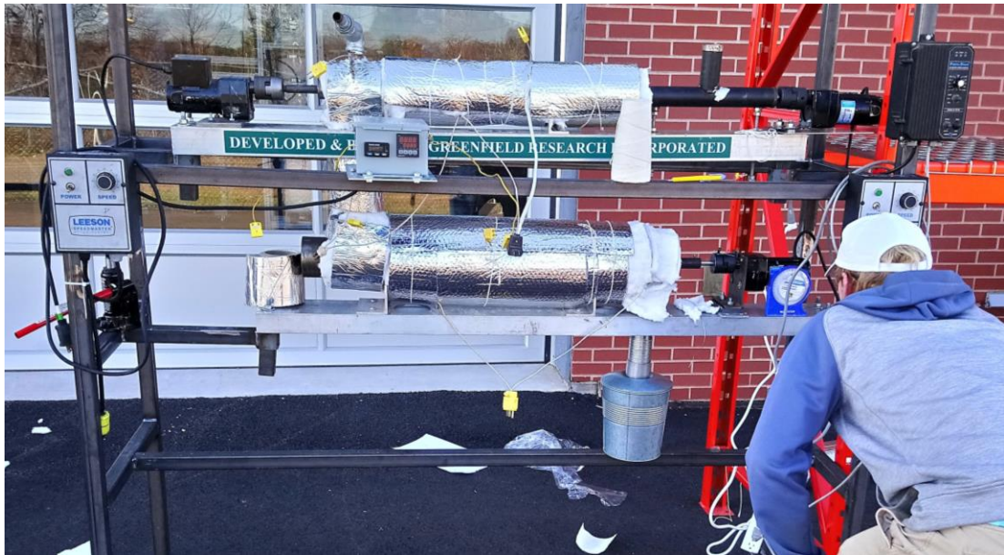
Two-stage rotating drum pyrolysis in operation.
