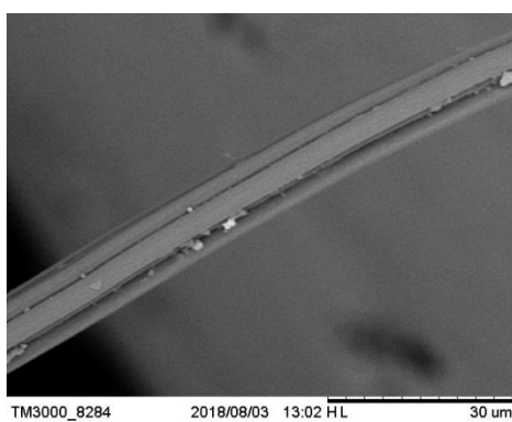
F-11. Fibrous particle with tube-like subunits.
