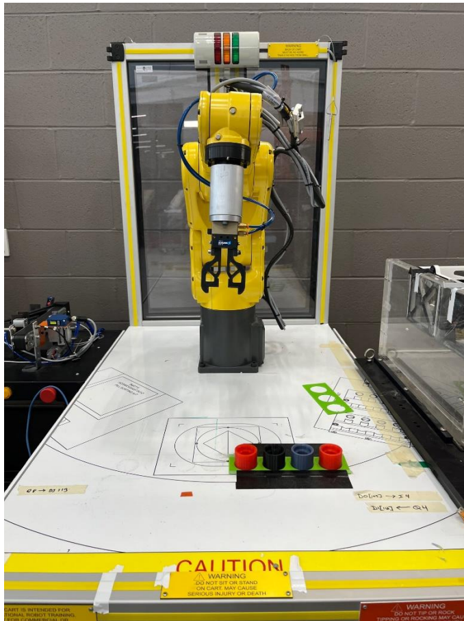
Figure 21: Photograph of the robotic arm used to pick up plastic samples.
