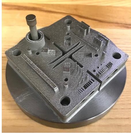
Figure 40: Successfully printed test artifact on the M100 build platform
