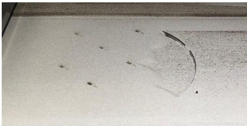
Figure 44: Underdosing observed for 40 \mu\text{m} print #2 on the M100
