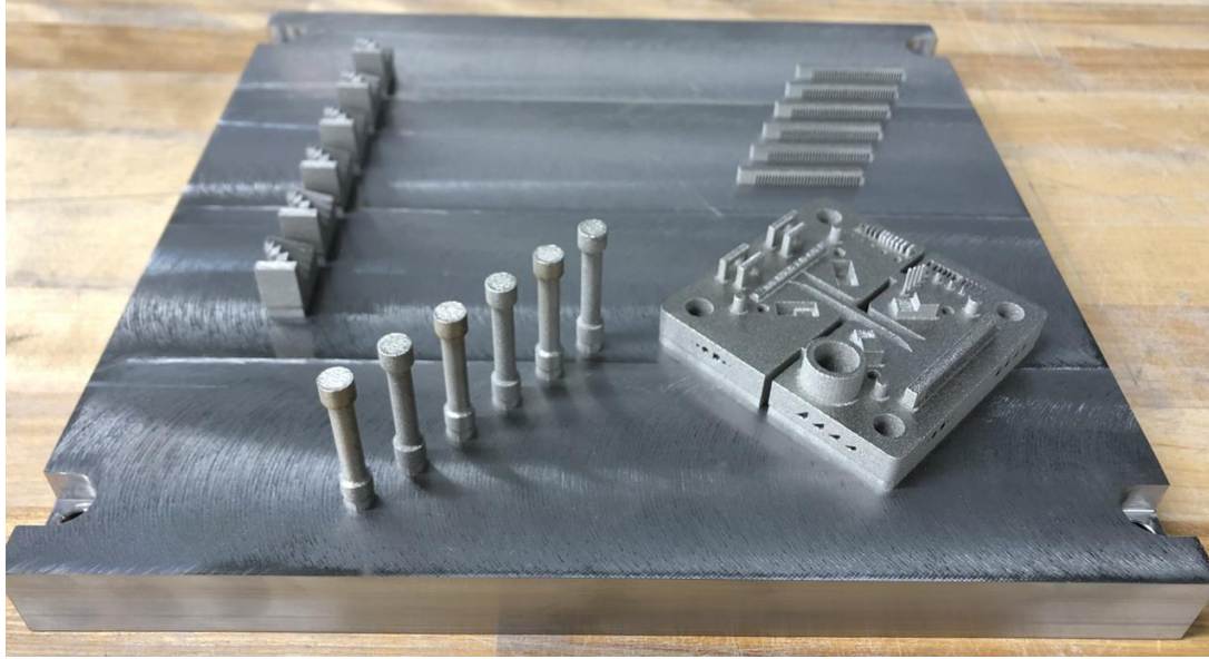
Figure 39: Final verification build printed on the M290
