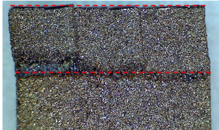
Figure 73: Image of a default-printed with nominal ledge thickness shown by the dashed red lines (ledge overhang length from left: 1 mm, 0.5 mm, and 0.25 mm)
