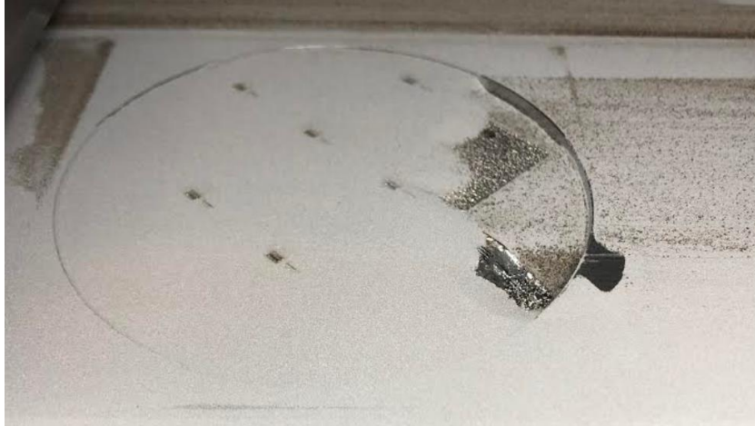
Figure 43: Underdosing observed for 40 \mu\text{m} print #1 on the M100
